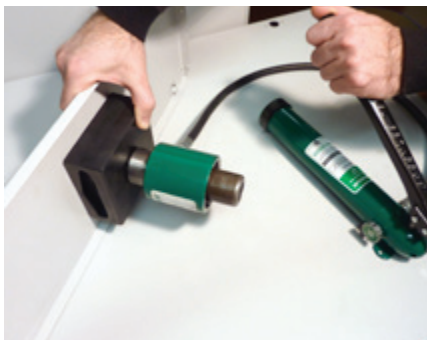
Making the cut-out with a punch
