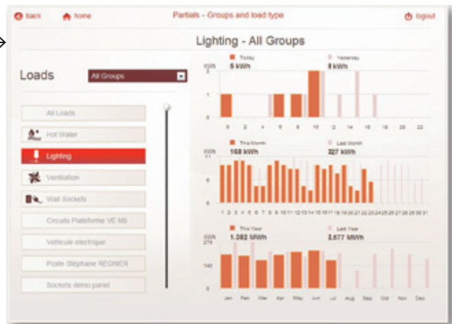
Display of consumption by circuit and measurement zone.
