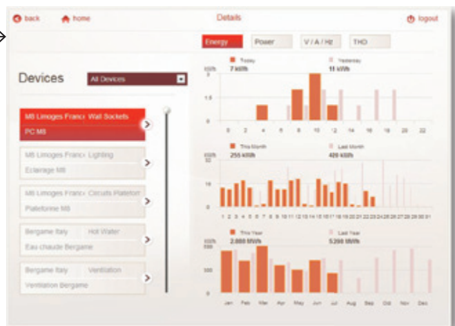
Display of consumption of each device according to the circuit or zone.
